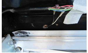
Further clean and straighten the extrusion and install the reinforcement part. Install as far forward as permits clearance between reinforcement and hinge bolts, and allowing access to turn jack-screw.
