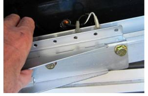
The wires are glued in place and the front corner of the extrusion is bent down on top of the wires. Straighten the front corner of the extrusion, free the glue with a sharpened narrow spatula, pull the wires free, and tape them out of the way:
