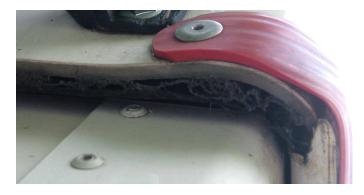
Here is an 18m ASH-26E metal trailer top, showing distorted front corner and rear latch miss-alignment.
